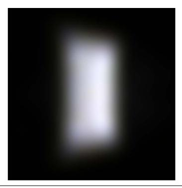
The Beam Pattern is rectangular (rectangle), good illumination uniformity, brightness difference is very little between the spot of center and periphery. Almost no difference in the direction of extending the road completely with the continuous extension of the road, it is the ideal lighting lamps for road lighting.
