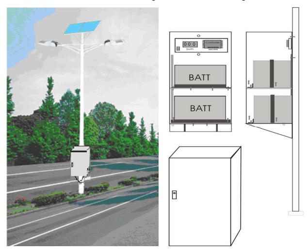
The Control Box Fixed on Lamp Pole Installation Diagram
